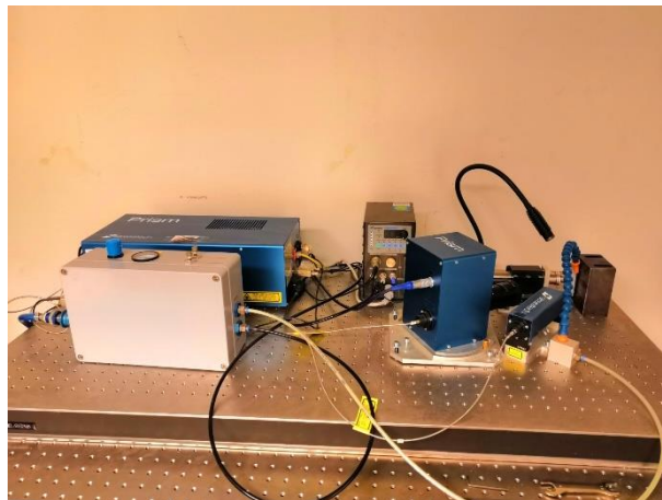
Figure 5. The residual stress device with hole drilling.
