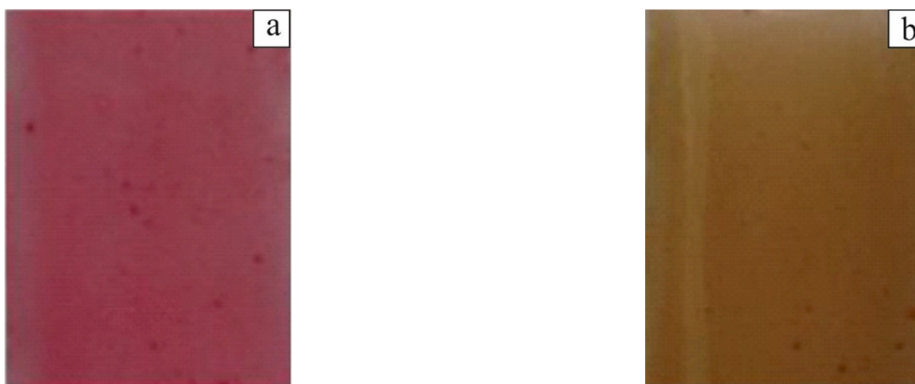
Fig. 9. Images of the as-prepared epoxy based coating filled with RhB loaded- \text{TiO}_2 containers (a) and UV irradiated during 60 min (b)
