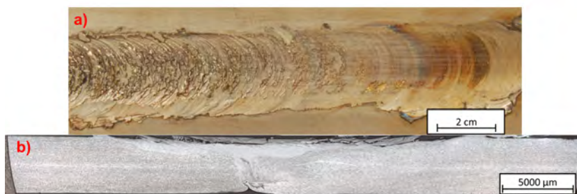
Fig. 7 Top (a) and Transverse (b) section for test 5 - 800 rpm, 1 mm/s and 35 kPa
