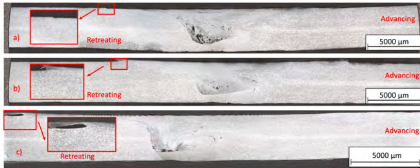
Fig. 9 Macrography results. a) Test 3 with Y = 26.27 , b) Test 4 with Y = 47.68 , and c) Test 1 with Y = 87.07 .
