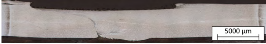
Fig. 8 Transverse section for Test 2 - 450 rpm, 1 mm/s and 50 KPa
