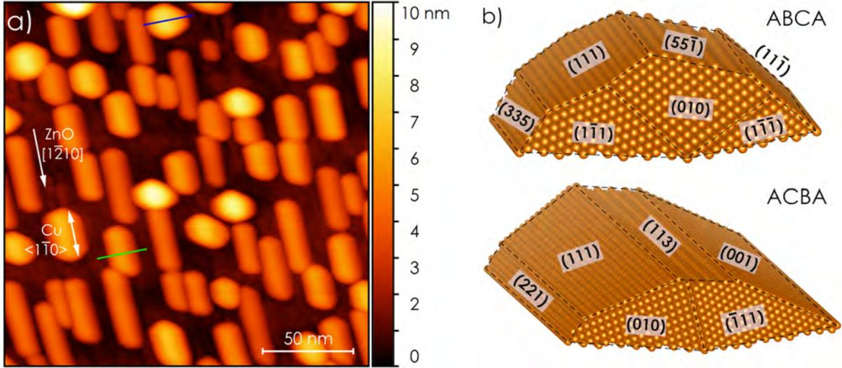
Figure 5: a) STM topography of Cu/ZnO(10 $\bar{1}$ 4). Indicated line scans over a ABCA (blue) and a ACBA (green) stacked NP correspond to Figure 6. The Cu[1 $\bar{1}$ 0] direction with respect to the ZnO[1 $\bar{2}$ 10] direction is parallel for ACBA stacked NPs, antiparallel for ABCA stacking order. b) Illustration of the NP morphology for both stacking variants.
