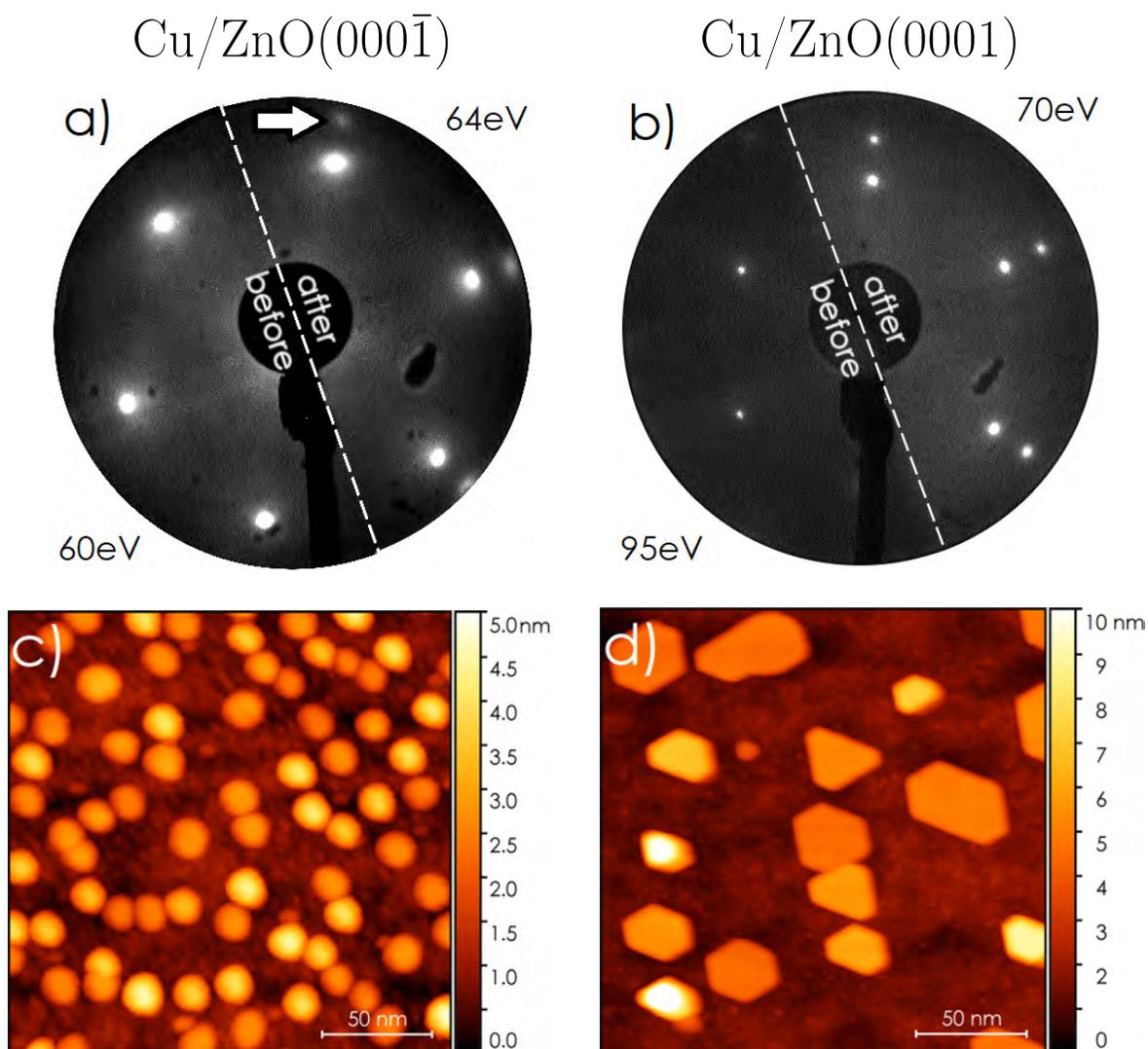
Figure 1: LEED images before and after Cu evaporation: **a)** ZnO(0001̄) and **b)** ZnO(0001). For better visibility, the contrast was individually adjusted and a white arrow was added to point out the position of a Cu reflection. STM topography measurements: **c)** Cu/ZnO(0001̄) and **d)** Cu/ZnO(0001). The NP height distribution statistics and SEM images of larger surface sections are available in the SI (Figures S1 and S2).
