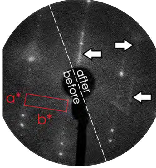
Figure 3: LEED images of ZnO( $10\bar{1}4$ ) before (left) and after (right) Cu growth ( $E_{\text{kin}} = 100$  eV). The arrow highlights the position of Cu signal, visible as a line. The red rectangle indicates the surface unit cell of the ZnO substrate with  $a = 2\pi/a^* = 12.4$  Å and  $b = 2\pi/b^* = 3.29$  Å.<sup>22,23</sup>
