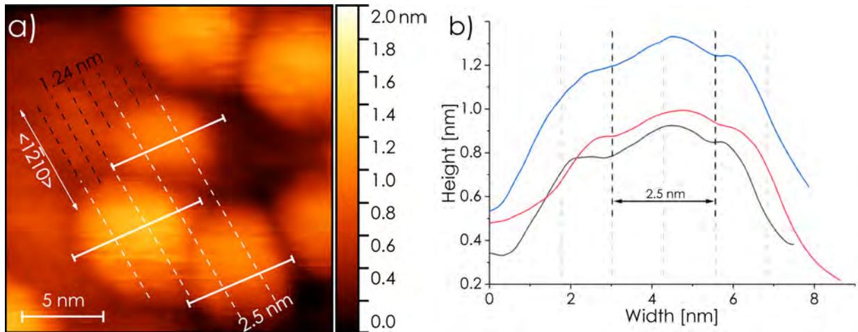
Figure 7: a) STM topography of 0.2 nm Cu on ZnO( $10\bar{1}4$ ). Black dashed lines indicate substrate step rows. b) Corresponding height profiles of the NPs in a). The line scans were translated horizontally to align the observed height depressions. Large area overview image available as Figure S3 in SI.
