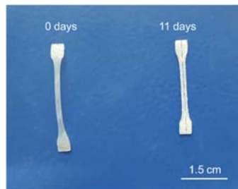
Figure 4. Standard test specimens, after programming and reversible actuation and 11 d after degradation.
