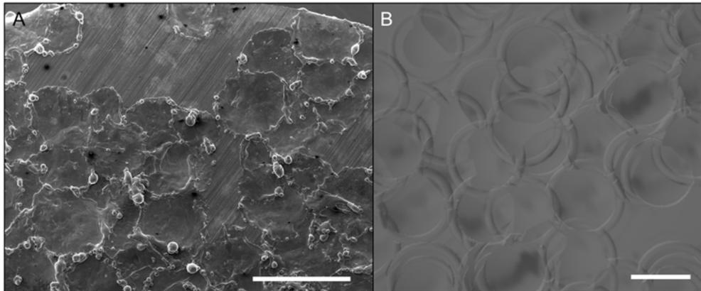
Figure 3 – A) A Scanning Electron Microscopy (SEM) image of a stainless steel EDM treated surface. Scale bar = 1000  $\mu\text{m}$ . B) A surface generated from simulation. Scale bar = 30  $\mu\text{m}$
