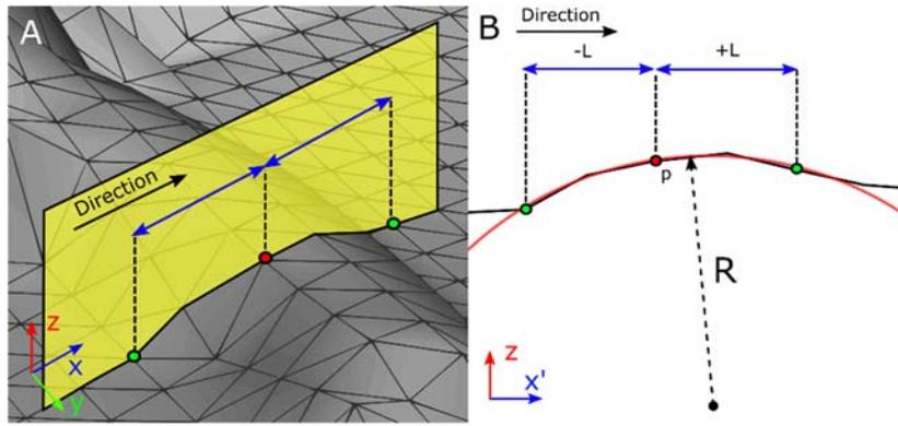
Figure 2 – Schematic of calculating curvature using 3 points on a 2D-plane and inscribing a circle on to it. For any three points  $\in \mathbb{R}^2$  there is only one unique solution to fit a circle. A) Looking at the selected points from the surface. B) Look at the selected points at the cut plane.
