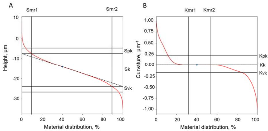
Figure 4. Abbott-Firestone roughness and curvature curves from a surface with the input  $a = 30 \mu\text{m}$  and  $h/a = 0.1$  after 5000 random impacts. The point at 40% material distribution shows at what point the tangential line is drawn, this in turn defined the parameter  $Sk$  and  $Kk$ . A) Abbott-Firestone roughness curve. B) Abbott-Firestone curvature curve
