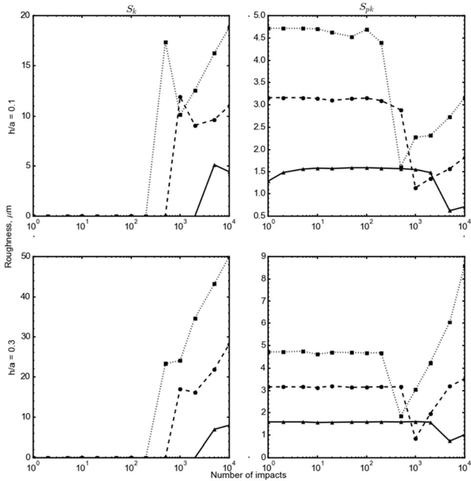
Figure 5 – Graphs of plotting  $S_k$ , core roughness profile (left), and  $S_{pk}$ , reduced peak height (right), as a function of number of impacts. Graphs with  $h/a = 0.1$  (top),  $h/a = 0.3$  (bottom). Lines are shown for impact radius,  $a$ , of  $10\ \mu\text{m}$  (line),  $20\ \mu\text{m}$  (dashed), and  $30\ \mu\text{m}$  (dotted).
