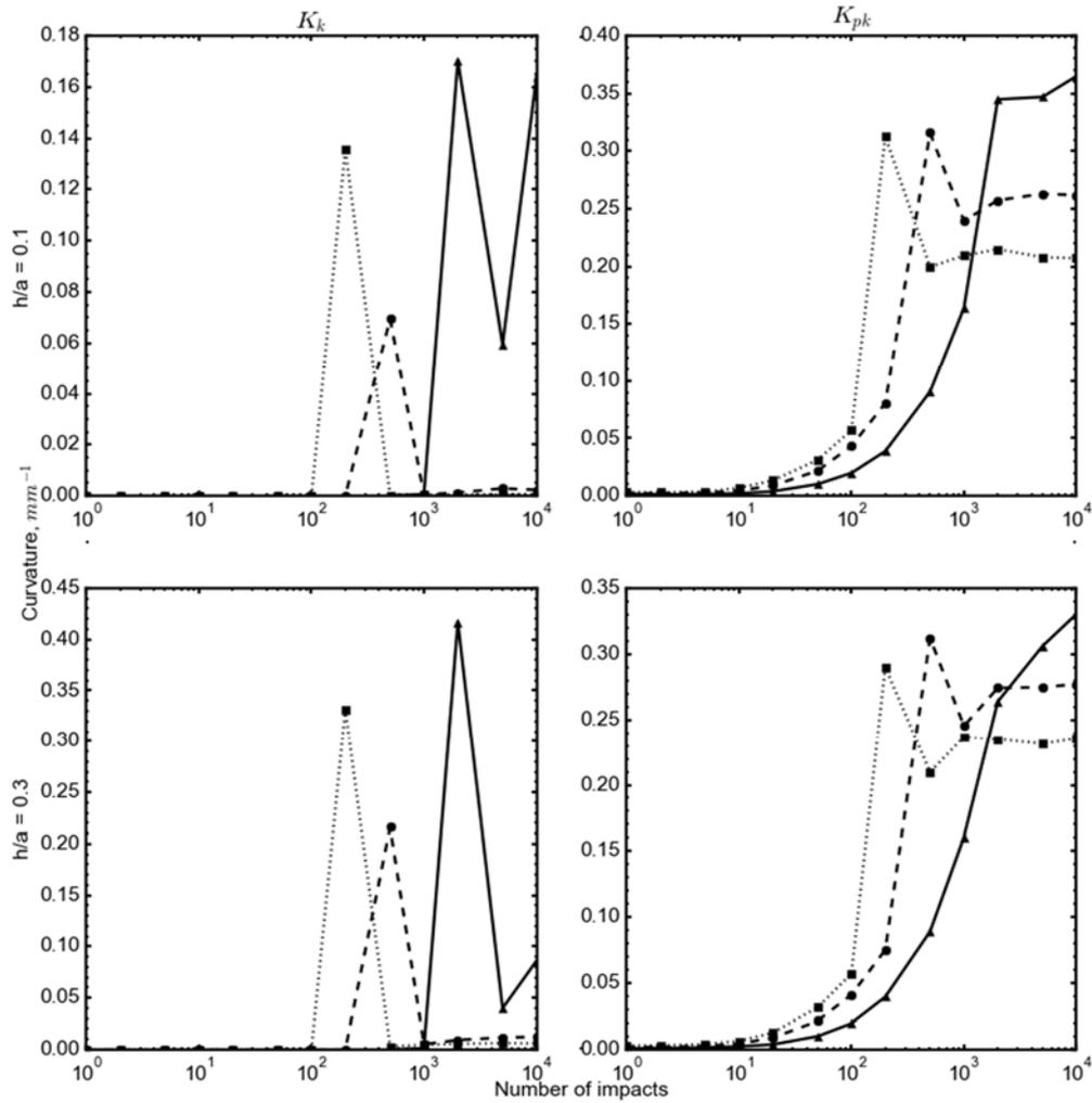
Figure 6 - Graphs of plotting  $K_k$ , core curvature profile (left), and  $K_{pk}$ , reduced curvature concavity profile (right), as a function of number of impacts. Graphs with  $h/a = 0.1$  (top),  $h/a = 0.3$  (bottom). Lines are shown for impact radius,  $a$ , of  $10 \mu\text{m}$  (line),  $20 \mu\text{m}$  (dashed), and  $30 \mu\text{m}$  (dotted).
