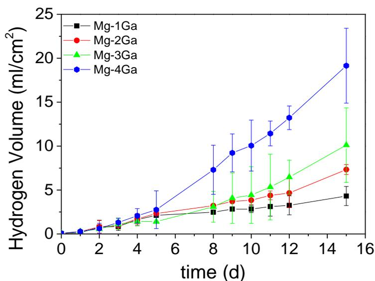
Figure 8. Hydrogen evolution measurements up to 15 days of immersion in NaCl 0.5 wt.% solution.
