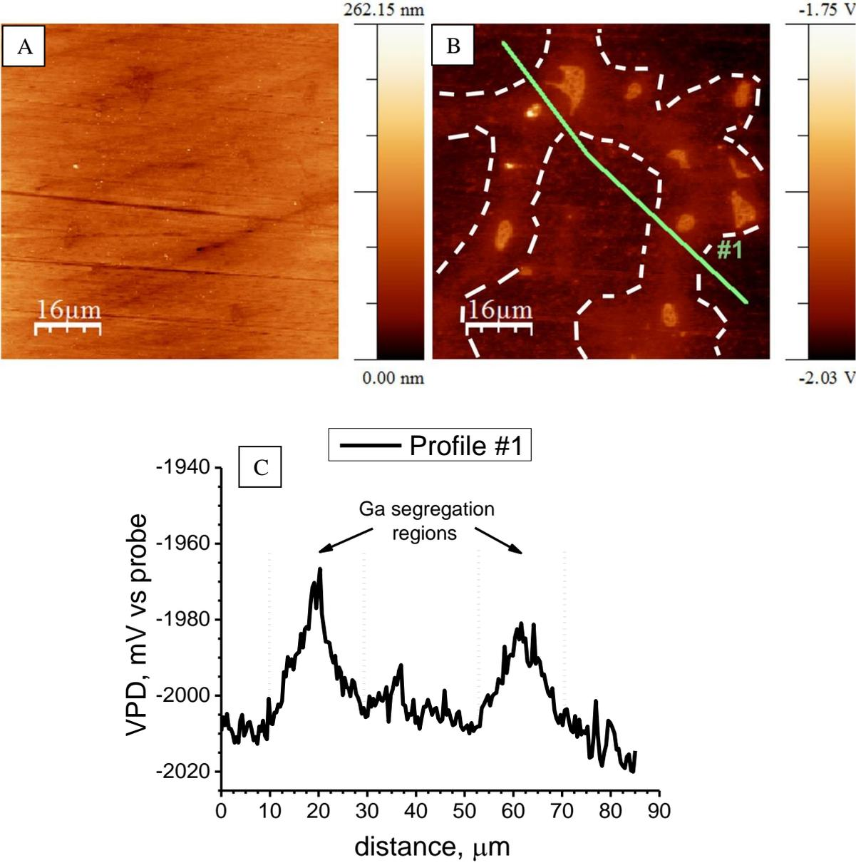
Figure 4. Mg-4Ga sample: (a) surface topography (b) SKPFM image and (c) VPD profile across the grain.
