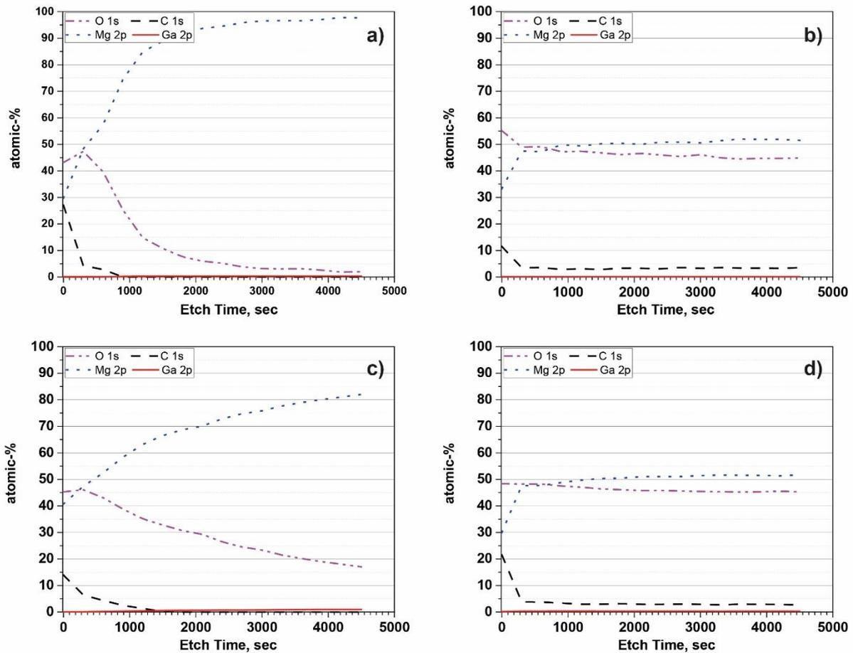
Figure 14. XPS depth profiles of (a) Mg-1Ga as-received (b) Mg-1Ga after exposure to electrolyte (EIS measurement) (c) Mg-4Ga as-received (d) Mg-4Ga after exposure to electrolyte (EIS measurement) (removal rate: 12 nm/min related to Ta<sub>2</sub>O<sub>5</sub>)
