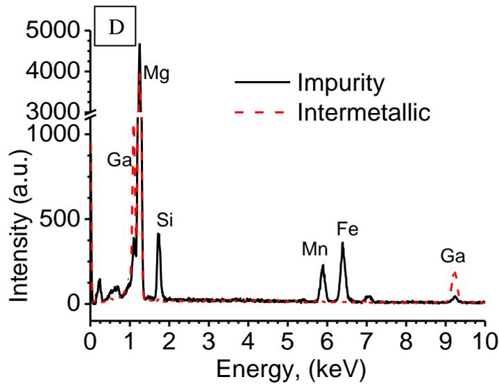
Figure 5. Mg-4Ga sample: (a) surface topography (b) SKPFM image and (c) and a VPD profile across the intermetallic and impurity; (d) EDS analysis of an impurity and intermetallic.
