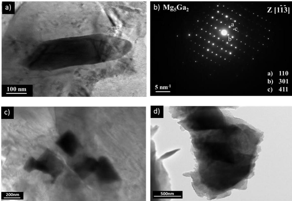
Figure 2. TEM analysis: (a) Second phase (b) electron diffraction pattern of the second phase (c,d) polygonal-shape particles containing impurities.
