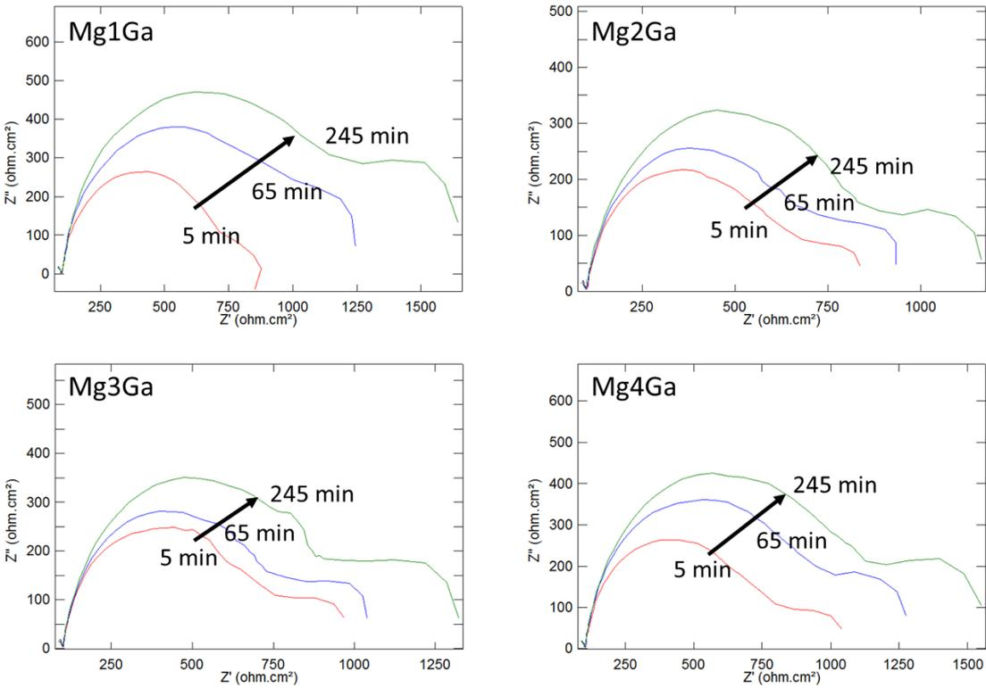
Figure 10. EIS measurements after potentiodynamic polarization in aerated 0.5% NaCl solution.
