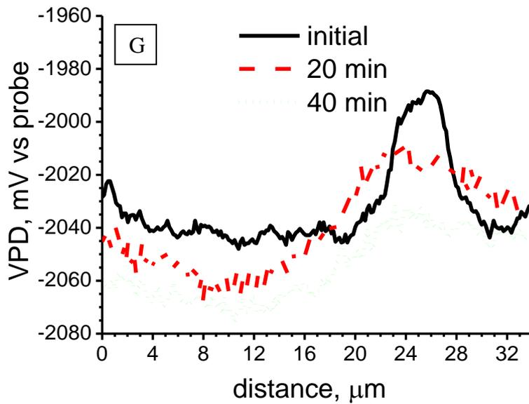
Figure 6. Mg-4Ga sample: (a,b,c) surface topography before and after immersion (20 and 40 min) in diluted NaCl solution, (d,e,f) SKPFM before and after immersion (20 and 40 min) in diluted NaCl solution (g) VPD profiles across the  $Mg_5Ga_2$  intermetallic.
