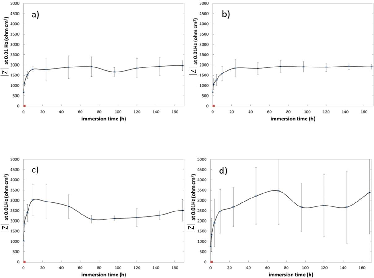
Figure 12. Development of low frequency impedance modulus values with immersion time of up to 168 hours in stirred aerated 0.5% NaCl solution for the different alloys a) Mg-1Ga, b) Mg-2Ga, c) Mg-3Ga and d) Mg-4Ga. The average values and the standard deviation (error bars) displayed are based on three measurements performed with three different specimens per alloy.
