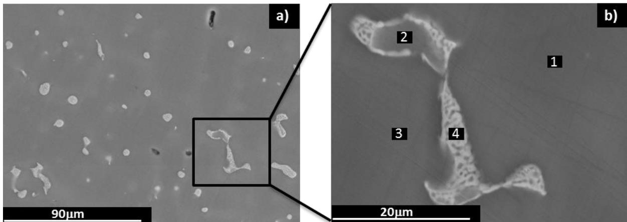
Figure 3. Scanning electron micrograph of the Mg-4Ga (a) lower magnification (b) a detail of the second phase  $Mg_5Ga_2$ .
