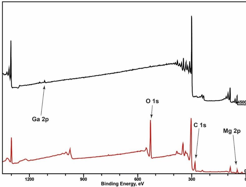
Figure 13. XPS survey spectra of Mg-1Ga as-received at 0 etching time (bottom) and after 4500 seconds (top).
