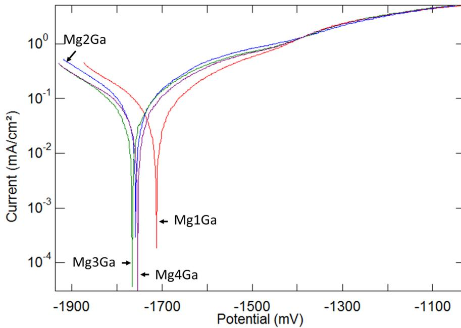
Figure 9. Polarization curves for the Mg-Ga alloys after 30 min of immersion in aerated and stirred neutral 0.5 wt.% NaCl solution.
