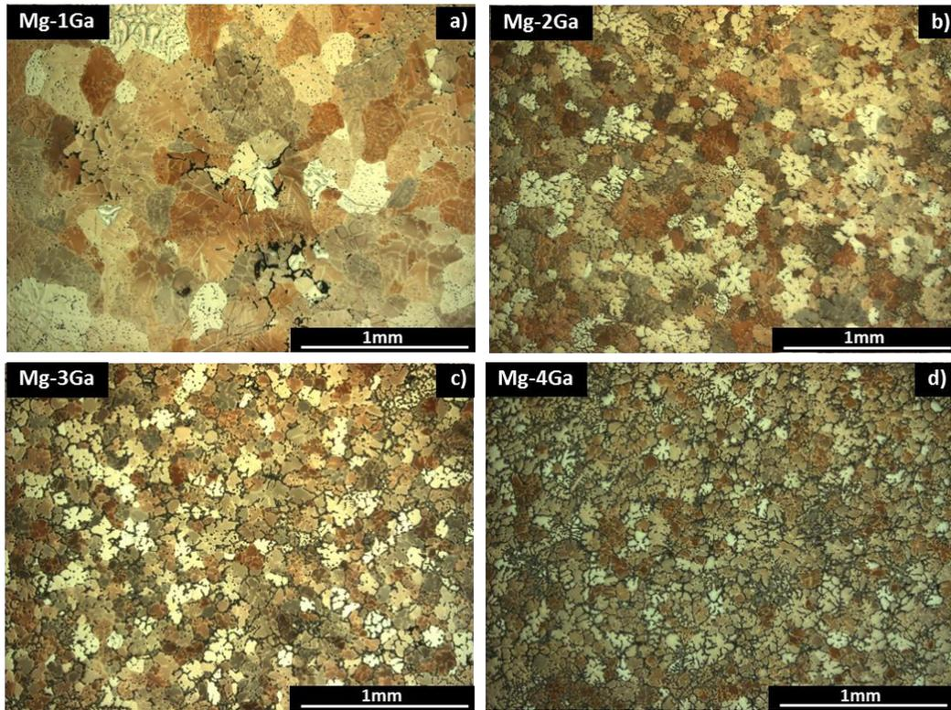
Figure 1. Optical micrographs of (a) Mg-1Ga, (b) Mg-2Ga, (c) Mg-3Ga and (d) Mg-4Ga alloys.
