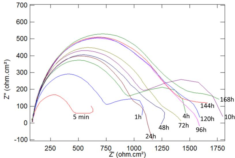
Figure 11. Typical impedance spectra for the alloys recorded during immersion in aerated 0.5% NaCl solution at RT. Example is showing the Mg-2Ga alloy with an early failure after 24 h immersion and slowly recovery of the protective film again.
