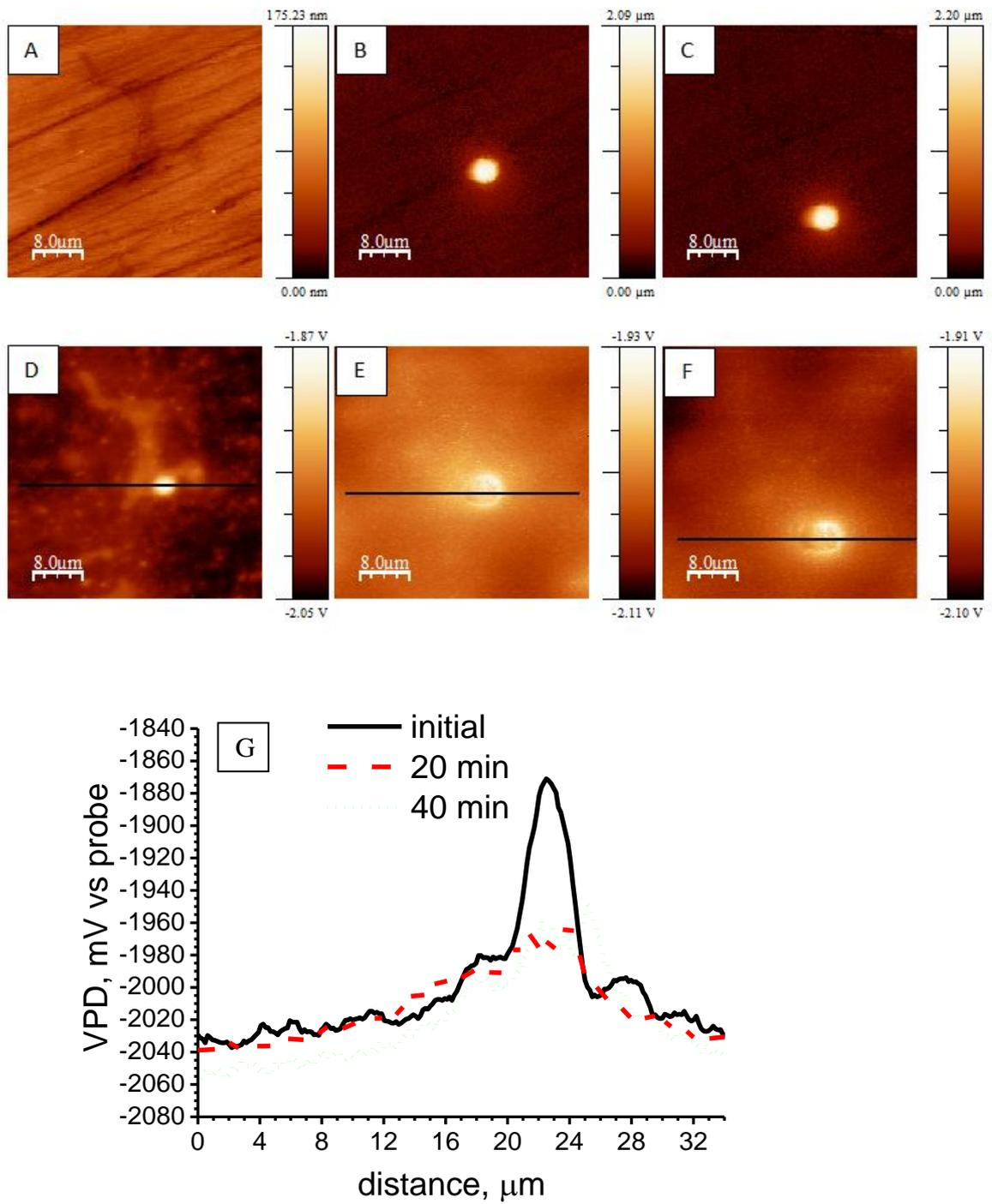
Figure 7. Mg-4Ga sample: (a,b,c) surface topography before and after immersion (20 and 40 min) in diluted NaCl solution, (d,e,f) SKPFM before and after immersion (20 and 40 min) in diluted NaCl solution (g) VPD profiles across the Mg<sub>5</sub>Ga<sub>2</sub> intermetallic and impurity.
