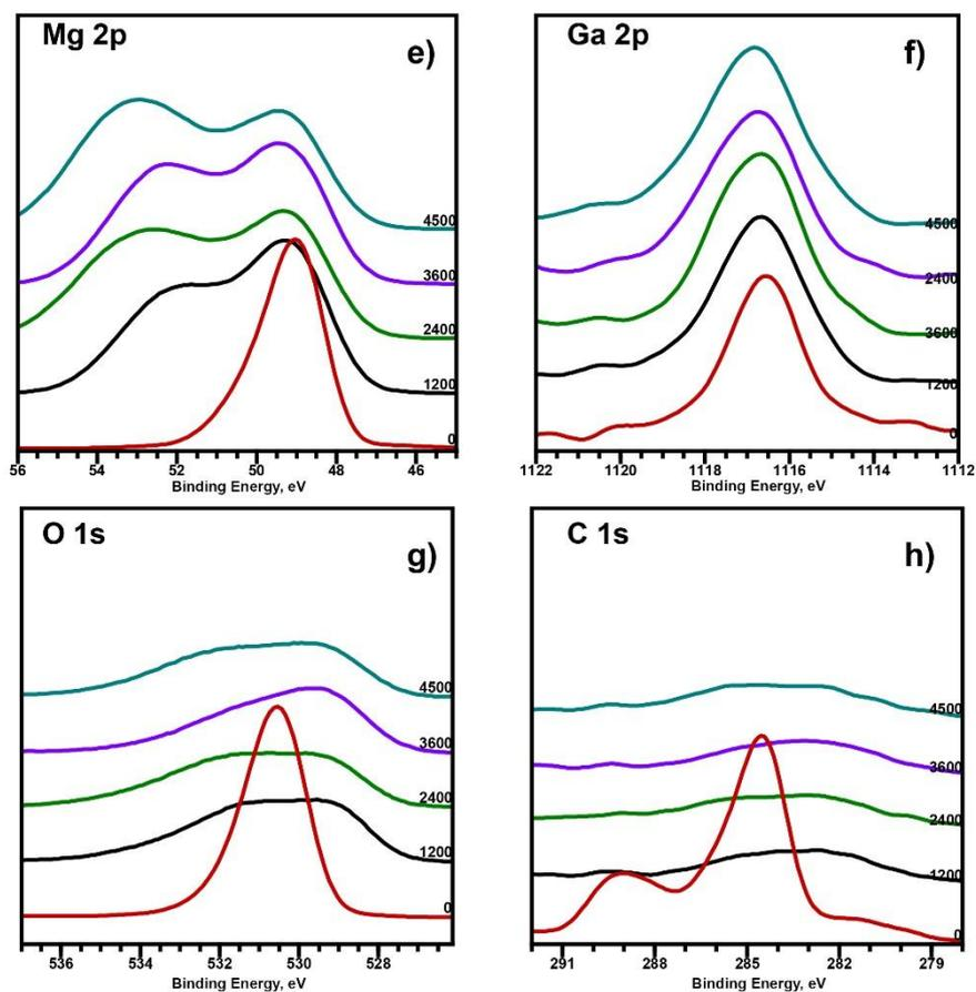
Figure 15. XPS regions for (a,b,c,d) Mg-1Ga as-received at 0 etching time and after 1200, 2400, 3600 and 4500 seconds and (e,f,g,h) Mg-1Ga after EIS measurements at 0 etching time and after 1200, 2400, 3600 and 4500 seconds.
