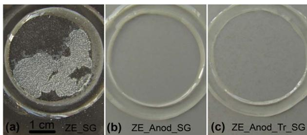
Fig. 5 Optical photographs of ZE\_SG after 7 days (a) and ZE\_Anod\_SG (b), ZE\_Anod\_Tr\_SG (c) samples after 30 days of immersion in 3% NaCl solution. The area exposed to the immersion test is 3.3 cm<sup>2</sup>.
