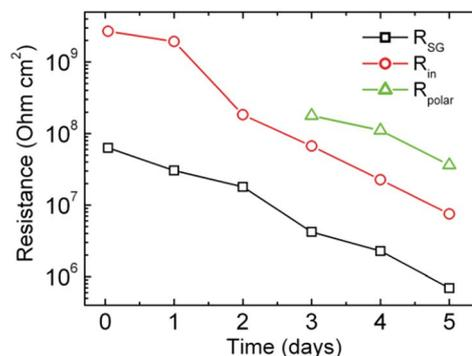
Fig. 4 Evolution of  $R_{\text{SG}}$ ,  $R_{\text{in}}$  and  $R_{\text{polar}}$  for ZE\_SG sample over the course of immersion in 3% NaCl solution.
