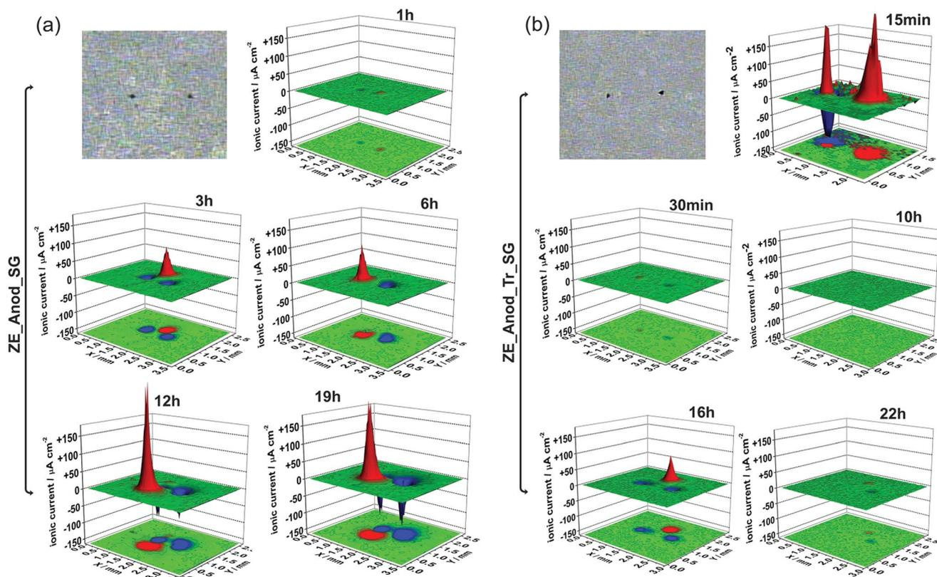
Fig. 8 Microphotographs of scanned area and distribution of ionic currents for **ZE\_Anod\_SG** (a) and **ZE\_Anod\_Tr\_SG** (b) after different immersion times in 0.05 M NaCl solution. The size of the scanned area shown in optical micrograph is  $2.7 \times 3.7$  mm.
