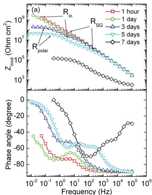
Fig. 3 Evolution of Bode plots for ZE\_SG sample in 3% NaCl (a) and equivalent circuits used for fitting experimental EIS spectra at different immersion times (b and c).
