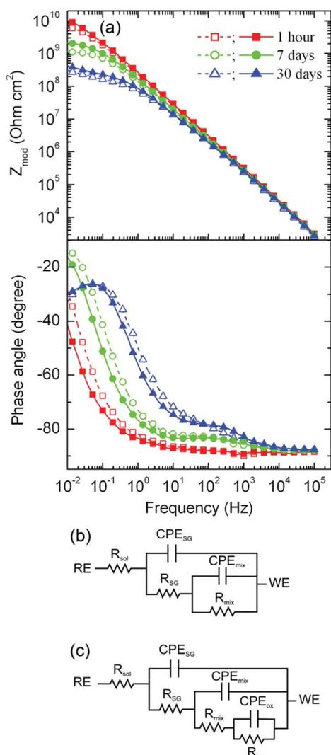
Fig. 6 Evolution of Bode plots (a) for ZE\_Anod\_SG (dashed lines, hollow marks) and ZE\_Anod\_Tr\_SG (solid lines, filled marks) samples in 3% NaCl; equivalent circuits used for fitting experimental EIS spectra at different immersion times (b and c).
