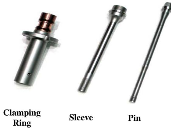
Fig. 1. Friction spot welding tool.
