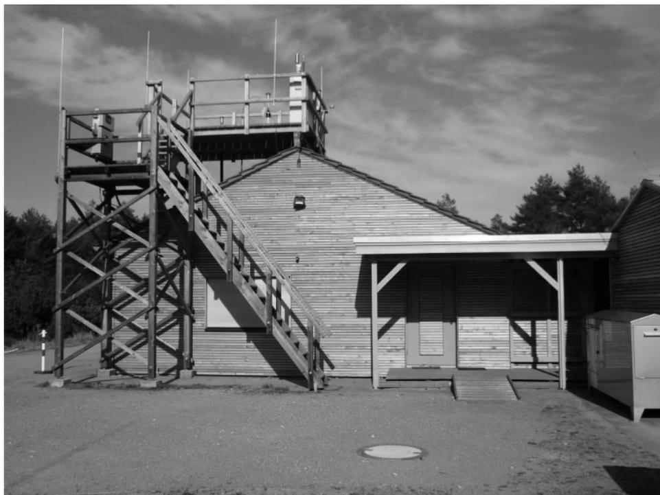
Fig. 1. Sampling tower with the equipment for speciated mercury measurements.
