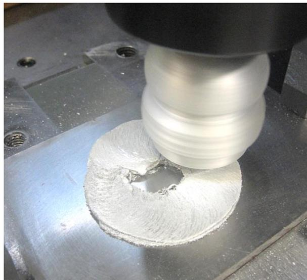
Fig. 45. Continuous AA6082-T6 build-up by FS along a 3D helicoidally trajectory (Vilaça et al., 2012).
