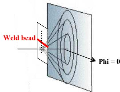
**Figure 1** – Schematics of the experimental setup for the laser weld structural analysis.
