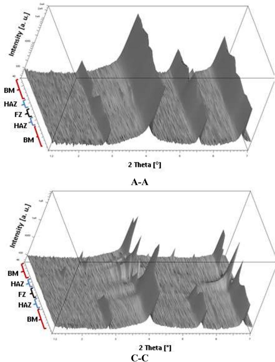
**Figure 2:-** X-ray diffraction patterns sequence along line scans across the laser weld bead.
