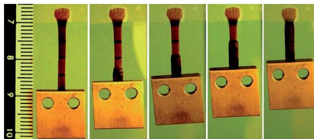
**Fig. 3** Photographs showing a spatially selective shape recovery process at room temperature by separate laser exposures on four sections of an AuNP-loaded XbOCL film stretched to 100% deformation (successively from the bottom section to the top section), with the film stepwise lifting a load 350 times its weight. Reproduced from ref. 33 with permission from The Royal Society of Chemistry.
