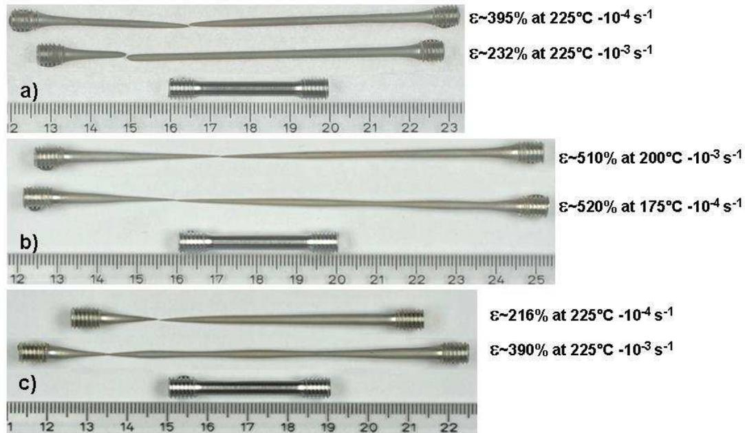
Fig. 4. Deformed samples in tension tested at different strain rates and temperatures for a) AZ31, b) AZ61 and c) AZ80.
