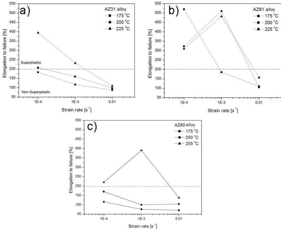
Fig. 3. Elongation to failure vs. strain rate for a) AZ31, b) AZ61 and c) AZ80 alloys tested at 175 °C, 200 °C, and 225 °C.
