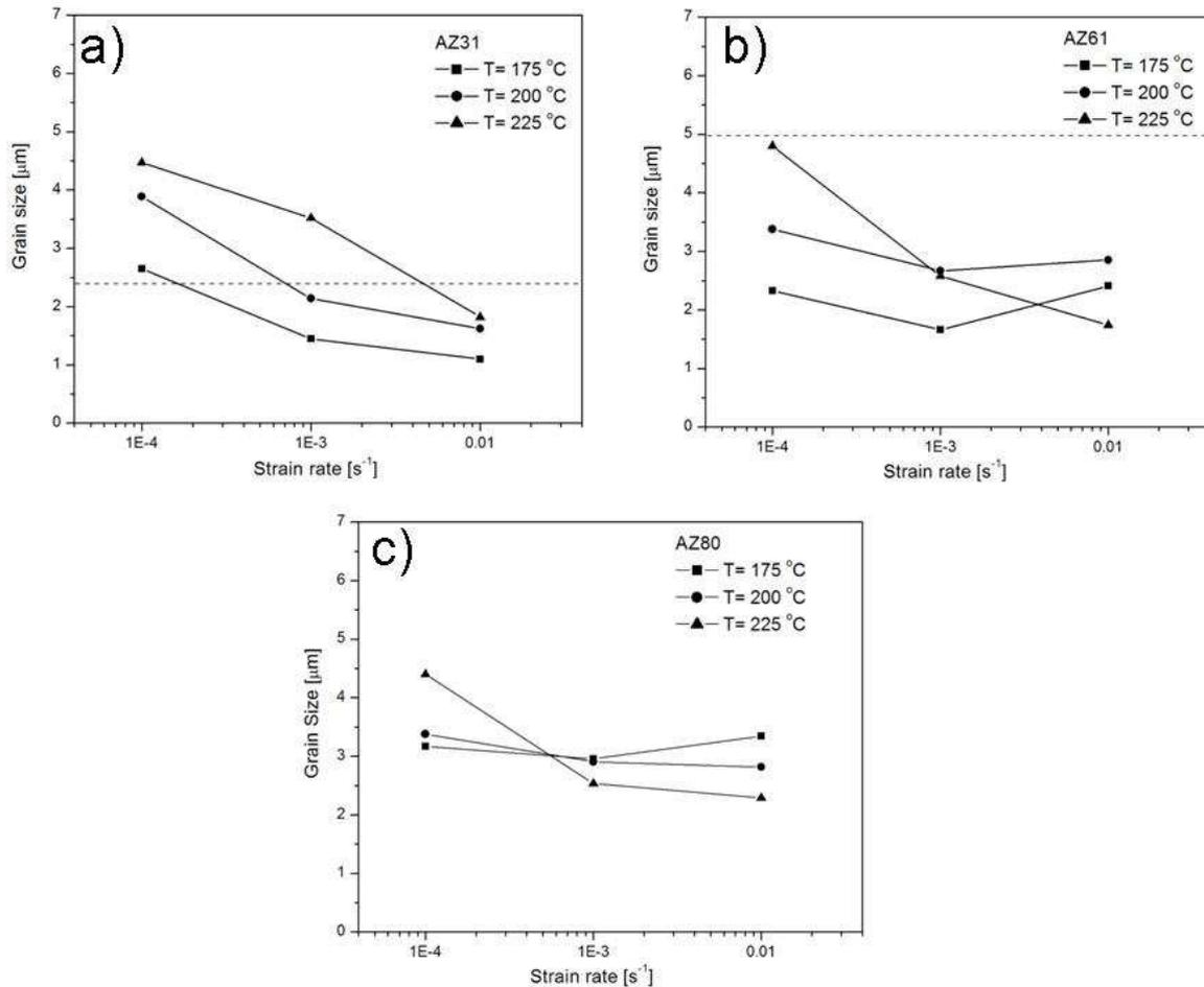
Fig. 5. Average grain size after deformation at different temperatures as a function of the strain rate a) for AZ31, b) for AZ61 and c) AZ80 alloy.
