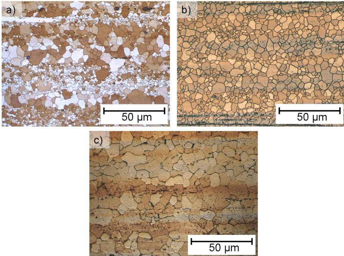
Fig. 1. Microstructure of hydrostatically extruded alloys a) AZ31, b) AZ61 and c) AZ80.
