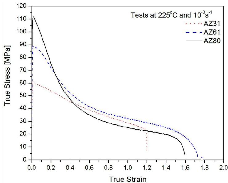
Fig. 2. True Stress-True Strain curves for all alloys tested at 225 °C and  $10^{-3} \text{ s}^{-1}$
