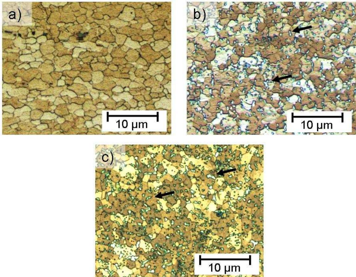
Fig. 6. Microstructures of samples deformed up to fracture at 225 °C and  $10^{-3} \text{ s}^{-1}$  for a) AZ31, b) AZ61 and c) AZ80 alloy.
