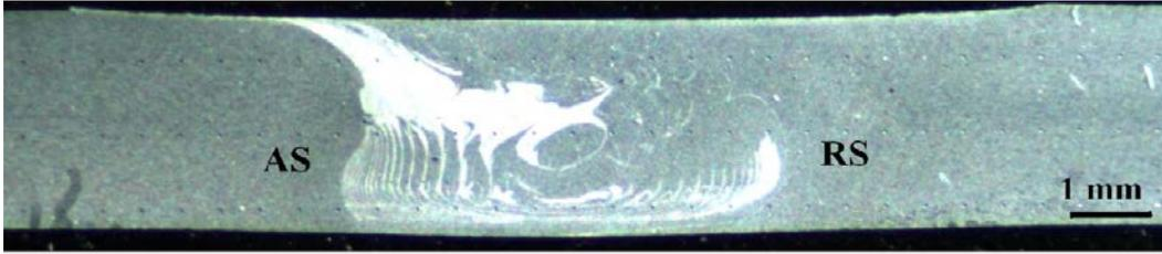
Figure 3 Macrostructure of a Friction stir welded joint in an Al 5083 alloy.
