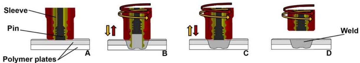
**Figure- 1- Illustration of the FSpW process: (A) to (D) the main steps with the Sleeve-Plunge variant.**
