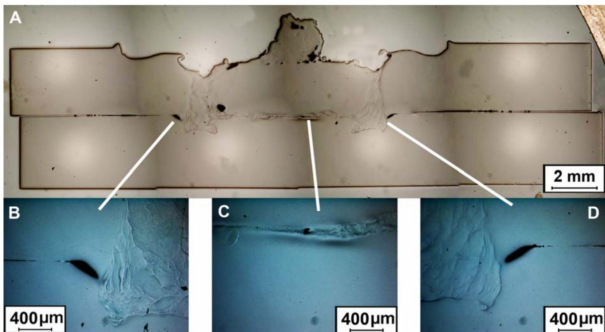
**Figure– 2 – Microstructure of a PMMA joint of FSpW (“sleeve plunge” at 500 rpm/ 5.5 s/ 3 bar/ 4 mm ): (A) Cross-sectional view from the weld center; (B) and (D) Details of the consolidated plasticized polymer; and (C) The central region of the spot, showing the bonding line between upper and lower plaques.**
