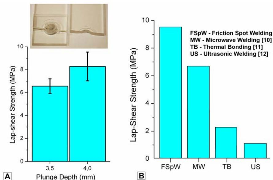
**Figure 4 – (A) average strength of PMMA FSpW joints (3 replicates) for two different plunge depths. An example of a fractured lap-shear specimen can be seen at the top of A; (B) Maximum weld strengths of PMMA joints welded by different techniques.**
