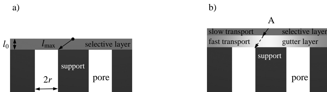
Figure 1 Simplified geometry of the composite membrane crosssection used for effective thickness derivation (a); introduction of gutter layer between support and selective layer (b)
