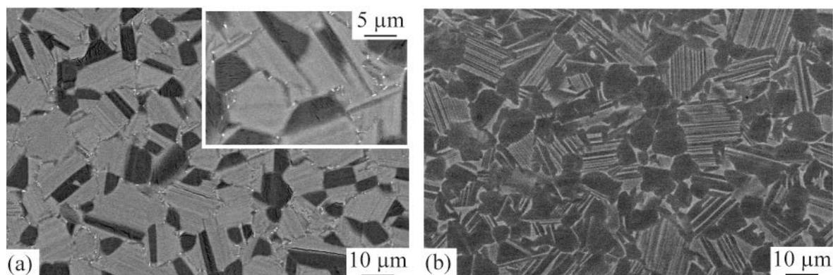
Fig. 2. Duplex microstructures of G4 and TNB alloys. (a) G4 alloy processed by SPS (1285°C, 2 min) and subsequently annealed in a furnace at 1320°C for 4 h. (b) TNB alloy annealed by SPS at 1290°C for 30 min.
