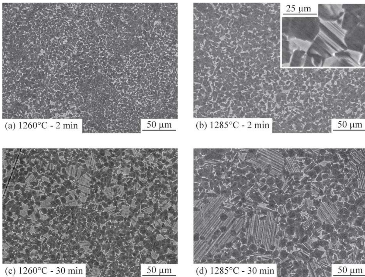
Fig. 1. Microstructures of the GE-SPS alloys processed at 1260°C and 1285°C for 2 to 30 min. Inset: higher magnification image of lamellar and  $\alpha_2$  grains.
