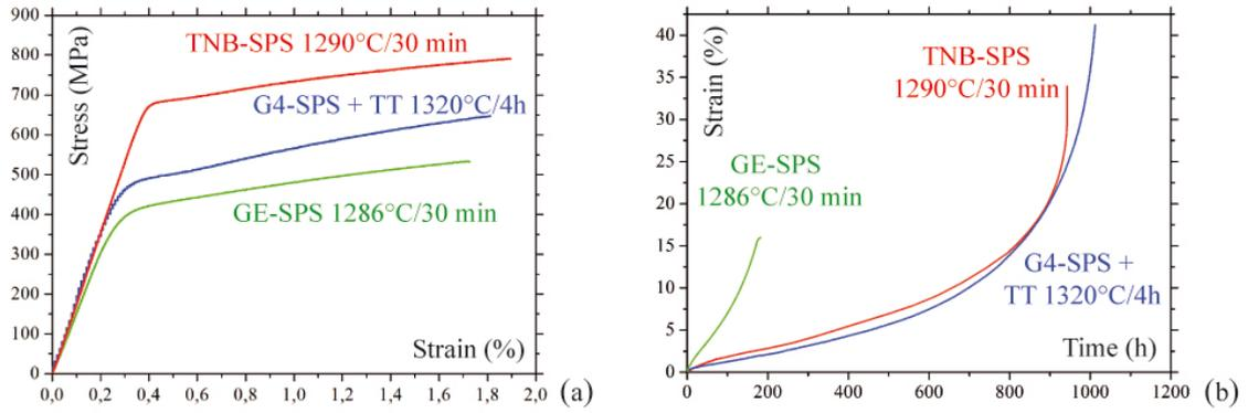
Fig. 3. Mechanical properties of duplex microstructures. (a) Room temperature tensile test curves, and (b) creep curves (700°C, 300 MPa) of the GE alloy processed by SPS at 1285°C for 30min, G4 alloy annealed in an external furnace at 1320°C for 4 h, and of the TNB alloy processed by SPS at 1290°C for 30 min.
