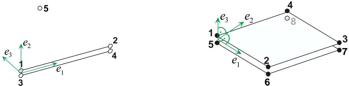
Figure 3: Cohesive elements for shell (left) and three-dimensional models (right).
